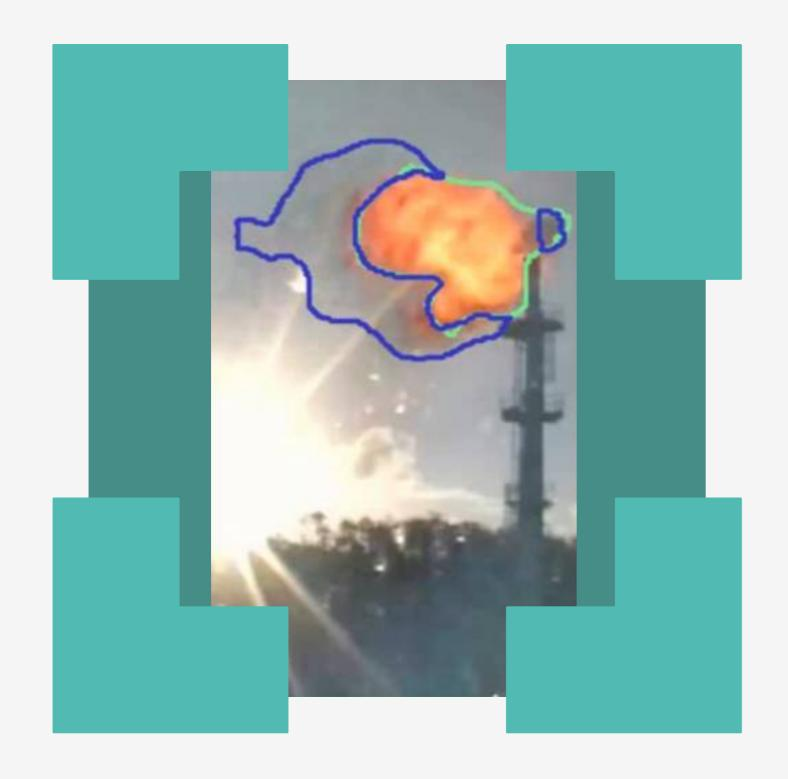
Noema's app automatically monitors gas flares for outages, while also quantifying the fire and smoke pixel-area. Operators get useful, real-time data and alarms to help reduce environmental impacts and regulatory costs.
